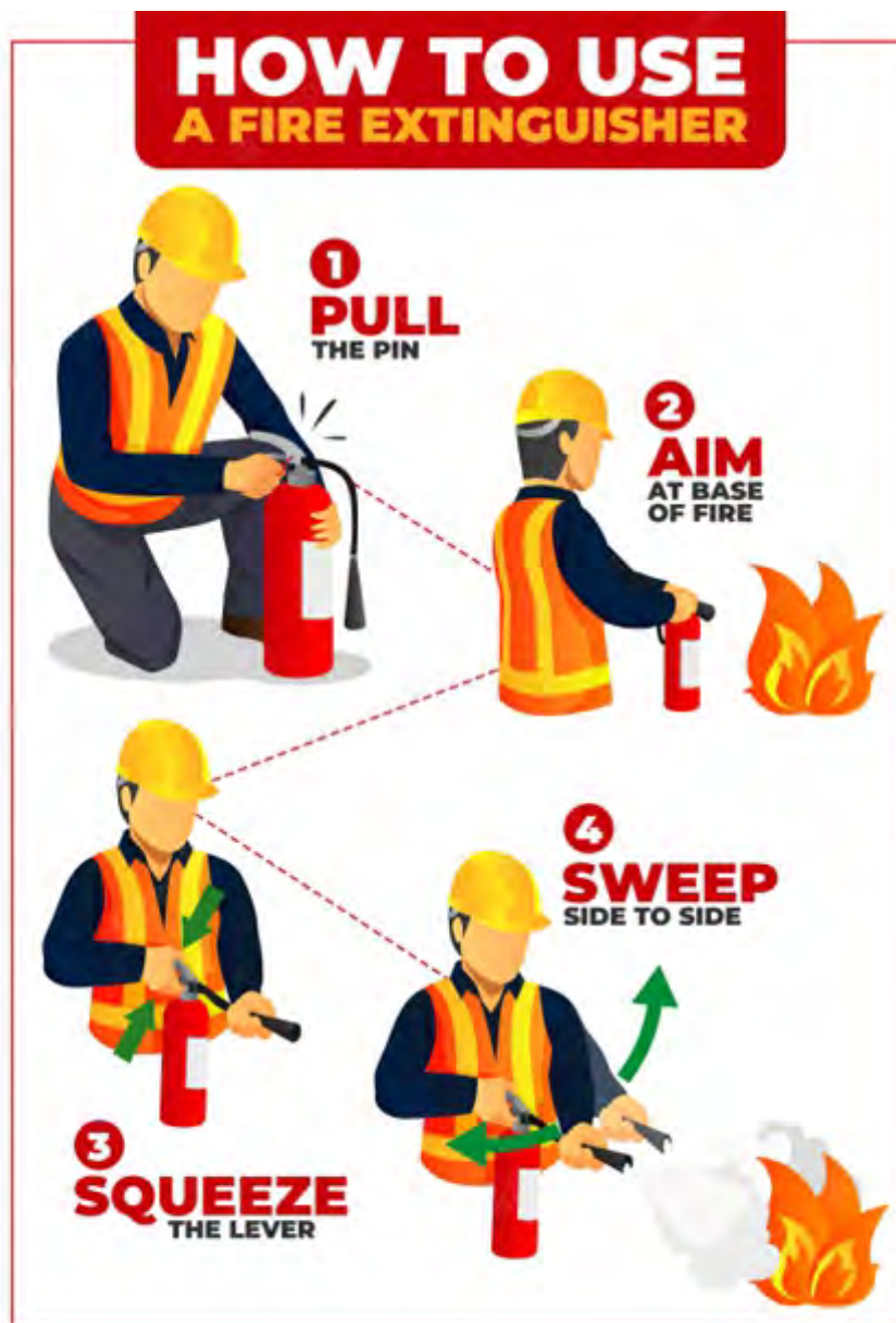
Fig. 5.1.13. Usage of Fire Extinguisher
